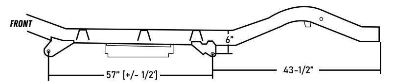
THESE ARE FACTORY STOCK TJ FRAME DIMENSIONS, THE EXACT LOCATION OF YOUR BODY AND TRAILING ARM MOUNTING HOLES MAY VARY SLIGHTLY.
