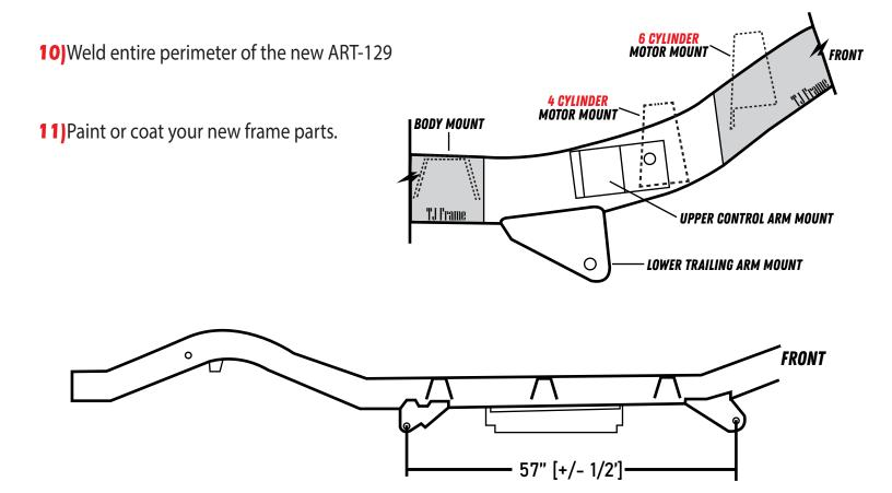
THESE ARE FACTORY STOCK TJ FRAME DIMENSIONS, THE EXACT LOCATION OF YOUR BODY AND TRAILING ARM MOUNTING HOLES MAY VARY SLIGHTLY.
