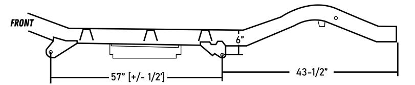
THESE ARE FACTORY STOCK TJ FRAME DIMENSIONS, THE EXACT LOCATION OF YOUR BODY AND TRAILING ARM MOUNTING HOLES MAY VARY SLIGHTLY.
