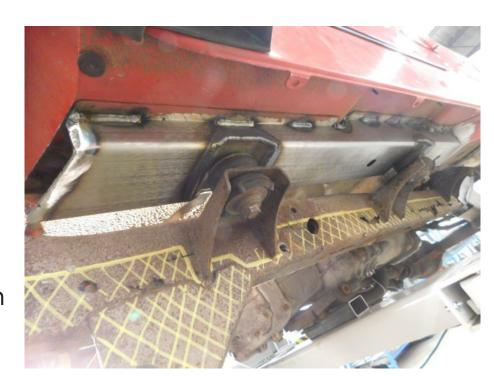
8) Seal seams with body seam sealer & paint. Reinstall all body mounts & torque to 50 ft-lbs.
