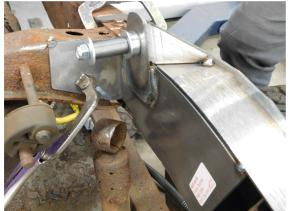
5) Place your kit against the upper and lower edges of the frame. The frame plate should sit firmly against the back side of the rear fuel tank crossmember.
