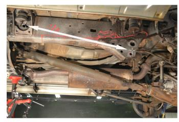
4) Cut the original control arm mount from the frame.
