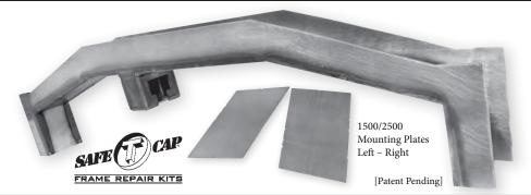
The ART-150 is designed to function like the original OEM crossmember, but does not resemble it in appearance.
