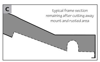
Use your new Safe-T-Cap<sup>TM</sup> as a guide and marker or chalk out a basic fit placement, keep a 1 inch minimum overlap of frame to Safe-T-Cap<sup>TM</sup>. Grind clean the remaining frame and rear crossmember attachment area, then position the Safe-T-Cap<sup>TM</sup> with measurements referenced in Illustration - A.
