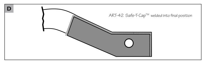
Fit Safe-T-Cap<sup>TM</sup> tightly up and back into frame. Measure again, tack weld corners in place. Once satisified with position and appearance, weld all edges 100% solid. Move the bead area around to avoid overheating.
