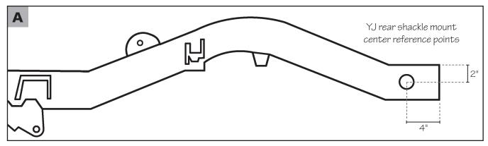
Start by measuring the distance center of the shackle mount to end of the rear crossmember, your frame may vary slightly from the factory specs above. Accurate measurements are key for factory correct alignment of your new Safe-T-Cap $^{TM}$  and proper suspension performance.
