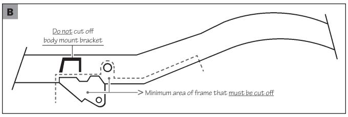
Use your new Safe-T-Cap $^{TM}$  as a guide and marker or chalk out a basic fit placement, then cut out frame 1 inch below the reference lines. Grind the remaining area clean and position the Safe-T-Cap $^{TM}$  in place with measurements referenced in Illustration - A.
