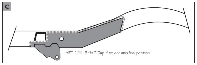
Fit Safe-T-Cap<sup>TM</sup> tight up into frame. Measure again and tack weld corners in place. Once satisified with position and appearance, weld all edges 100% solid. Move the bead area around to avoid overheating.
