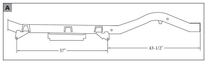
Start by measuring the distance between holes centers of the front and rear trailing arm mounts, be as accurate as possible and record for exact fit. These measurements are key for factory correct alignment of your new Safe-T-Cap $^{\text{TM}}$  and proper suspension performance.
