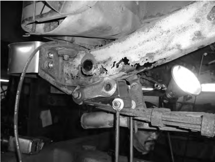
rusty frame section before repairs
