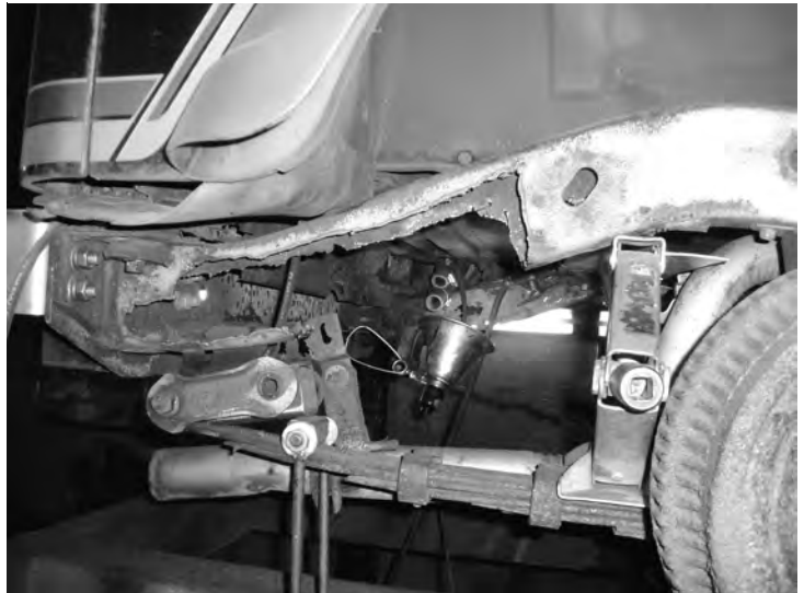
steel sleeve removed and rust cut back note we leave the top in place to help maintain the original alignment
