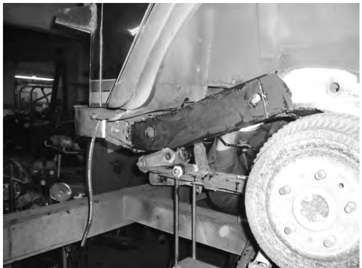
repairs primed and ready for undercoating
