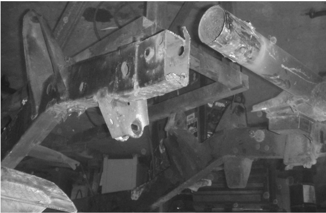
Figure C shows the front radiator support left in place
