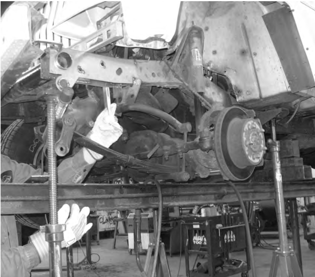
Figure D shows us leveling and adjusting the frame repair kit
